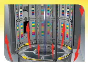
Air Flow in Test Chamber
