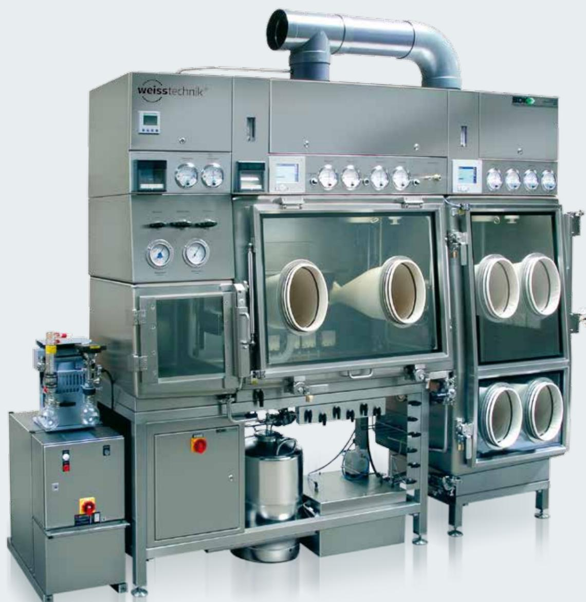
Insulators can be used anywhere where a controlled atmosphere needs to be created away from the installation room. In addition, they offer optimal protection for products and employees. Depending on the area of application, insulators are operated at underpressure for protection of persons and the surrounding area and at overpressure when solely providing product protection.
