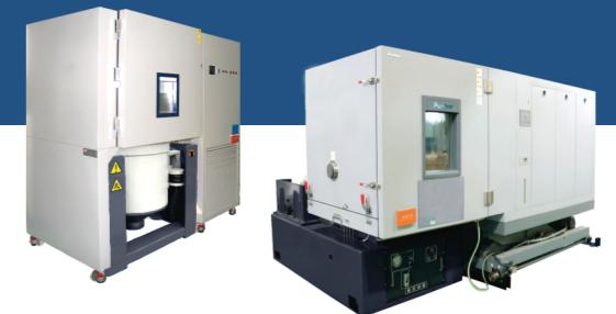
The integrated environmental testing system is designed to simultaneously test temperature, humidity and vibration. The test system provides the ability to define and perform tests for each of these elements at the same time. This system is widely used in reliability tests, identification tests and stress screening and often incorporates rapid temperature changes.
